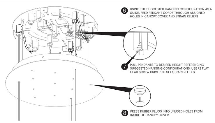
NOTE: INSTALLATION SHOWN IS FOR SOLIS CHANDELIER 3. FOR SOLIS CHANDELIER 5, FOLLOW THE SAME WIRING PROCESS USING THE HOLE PLACEMENT OUTLINED IN SUGGESTED HANGING CONFIGURATIONS
